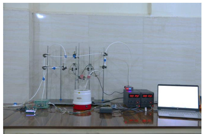
Figure 1: Experimental characterization platform for vapor delivery, sensor-chamber exposure, and data acquisition.
